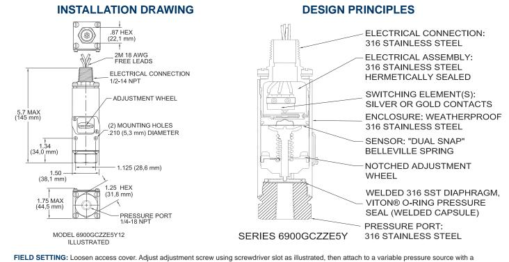
suitable gage, and check that the circuit continuity operates at the pressures desired. Clockwise to increase settings. Counterclockwise to decrease setting.
